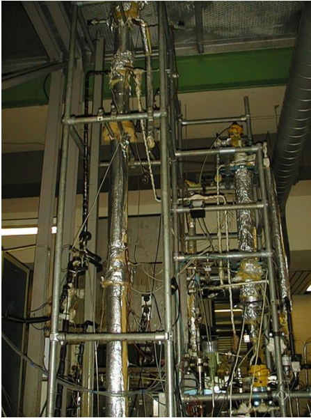
Figure 4 : Countercurrent SFE plant, and basic process design (Brunner, 1994)
