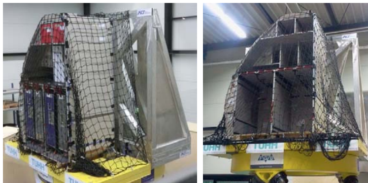
Figure 11: An A320 Aircraft galley G2 on the Hexapod test rig
