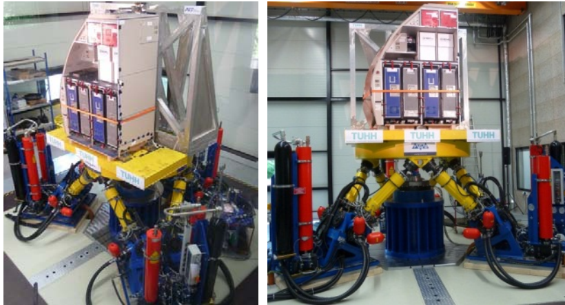
Figure 1: Aircraft Galley on the Hexapod test rig.
