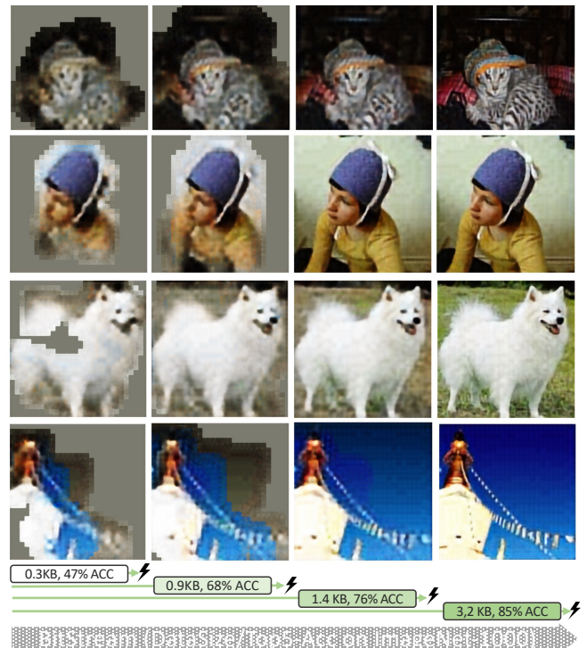
Figure 1: Qualitative comparison of LimitNet 's progressive reconstruction. LimitNet detects the important parts of the image and sends the encoded data in the order of importance. Progressive offloading allows the cloud to run the inference at any point (lightning symbol). The horizontal axis shows the offloading bitstream of an image, the first number shows the size of received data (in KB) at a specific time, followed by the corresponding Top5 Accuracy (Top5-Acc) of EfficientNet-B0 [61] on ImageNet1000 [27] using this received data.
